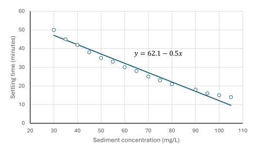
d. Settling time when the sediment concentration is 130 mg/L.
