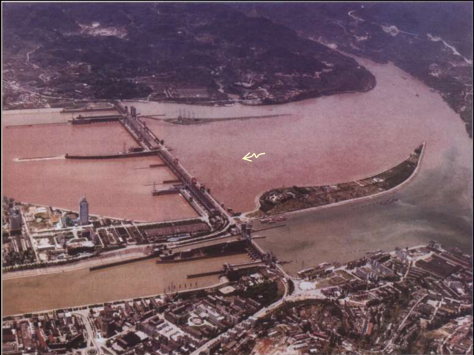
Fig. 6. The Three Gorges layout is based on the Gezhouba dam, built 20 years ago, and 38 km downstream
